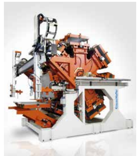
Drum unit equipped with two robotically manipulated mixing heads to enable quick filling of doors for increased productivity.
