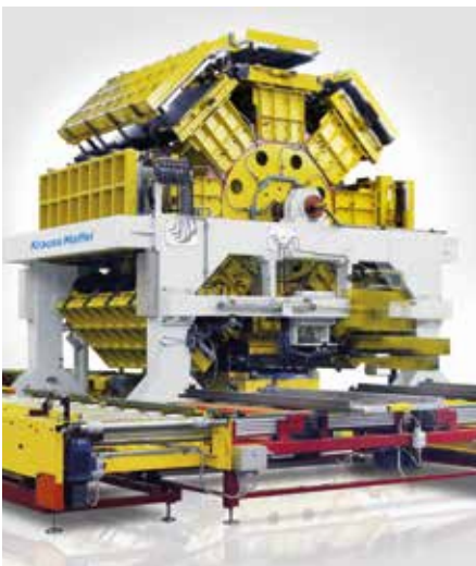
8-station drum technology for closed-mold foaming of doors
